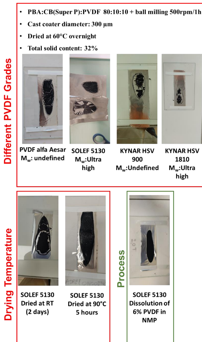
Figure 18. Image of the PBA formulated at 80:10:10 (PBA:CB:PVDF) using different PVDF types (Alfa Aesar, Solef 5130, Kynar HSV 900, and Kynar HSV 1810), employing different drying temperatures (25°C over 2 days and 90°C over 5 hours), and altering the process by diluting 6% PVDF by weight in NMP (Targeted Loading 8 mg cm -2 ).
